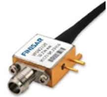
The VPDV2120 (Order Code VPDV2120-VF-FA) is not matched to 50 Ω and requires a bias voltage of -6 V, for which an external Bias-Tee (Order Code EVAL KIT VPDV) can also be ordered.
