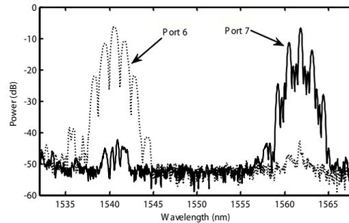
Figure 5: Spectral intensity response measured on two different output ports of the WaveShaper 4000E respectively the profiles of a 2-pulse burst at 1541 nm and a 4-pulse burst at 1562 nm
