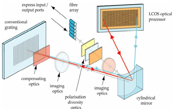
Figure 2: Schematic layout of the WaveShaper 4000E
