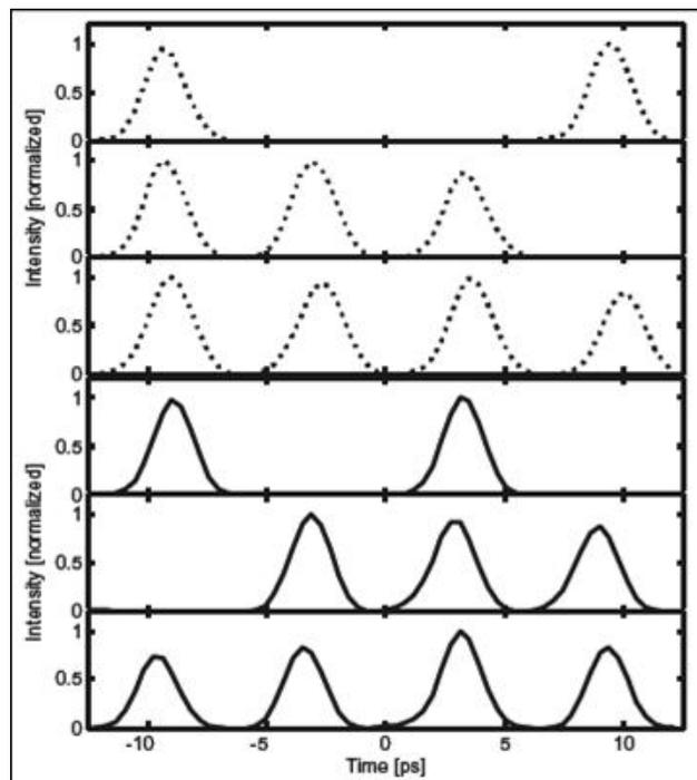
Figure 6: Measured temporal intensity profiles of various pulse bursts around a carrier wavelength of 1562 nm, sent to output port 1 (top three) of the WaveShaper 4000E and around 1541 nm sent to output port 2 (lower three).
