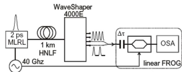
Figure 4: Experimental layout. MLRL = mode-locked ring laser; HNLF = highly nonlinear fiber; OSA = optical spectrum analyzer; FROG = frequency resolved optical gating.
