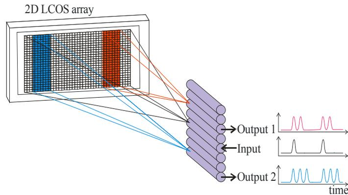
Figure 3: Schematic overview of how different parts of the LCoS can act on different parts of the spectrum. The blue part is programmed to re-shape a short input pulse into a pulse burst with three pulses, and send this specific wavelength range to 'Output 2' whereas the red part is programmed to reshape a short input pulse into a burst of 2 pulses that are being sent to 'Output 1'.
