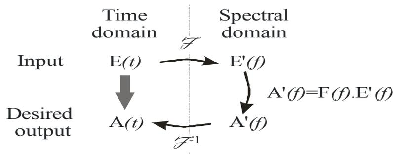
Figure 1: Schematic representation of Fourier-domain pulse shaping.
