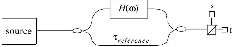
Figure 6. A Mach-Zehnder set-up for interferometric characterization of optical components using polarization diversity detection.
