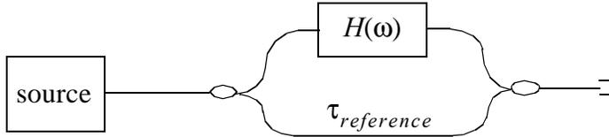
Figure 2. Basic Mach-Zehnder set-up for interferometric characterization of optical components. If a broadband source is used and  $\tau_{reference}$  is varied, then  $h(t)$  is measured in a technique known as Optical Low Coherence Reflectometry (OLCR). If  $\tau_{reference}$  is held constant, and the source is a scanning tunable laser, then  $H(\omega)$  is measured in a technique known as Optical Frequency Domain Reflectometry (OFDR)
