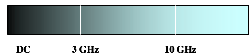
Figure 1. Direct modulation (dark background) is used almost exclusively through 3 GHz, and overlaps with external modulation (light background) between 3 and 12 GHz. External modulation is necessary above about 12 GHz.
