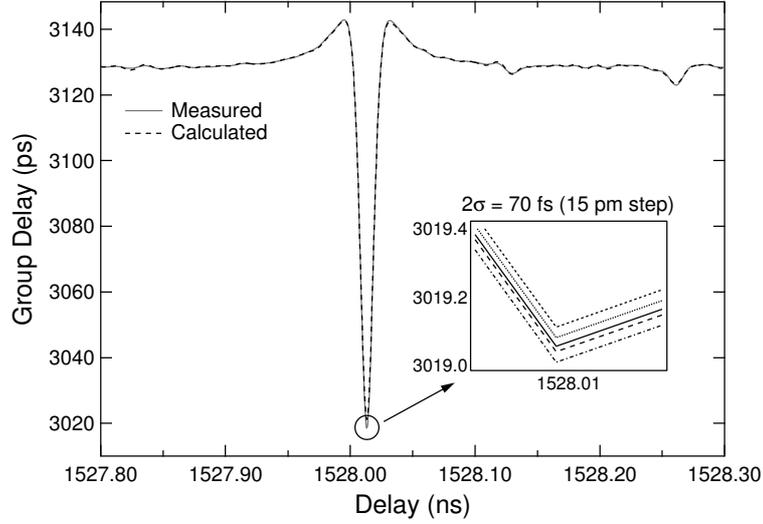
Figure 3: Group delay of an Acetylene gas cell as measured (solid) using the technique described in this paper and as calculated (dashed) from the loss of the same cell. The inset shows five representative data sets illustrating measurement repeatability.
