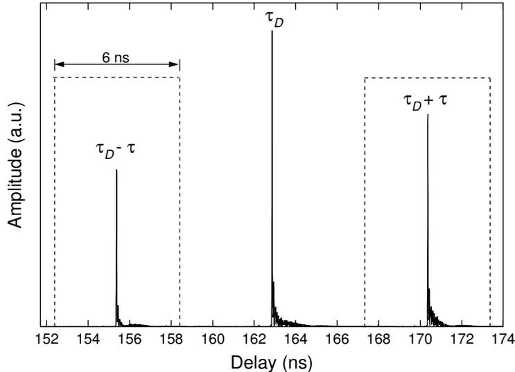
Figure 2: Discrete Fourier transform of raw data from one of the two detectors, S and P. The DUT was a Bragg grating. The peaks at  $\tau_D - \tau$  and  $\tau_D + \tau$  are associated with two elements of the DUT TF. The dashed boxes represent bandpass filters used to “slice out” these impulses in order to extract the DUT TF elements. The 6 ns width of these filters limits the measurable GD or PMD to 6 ns.
