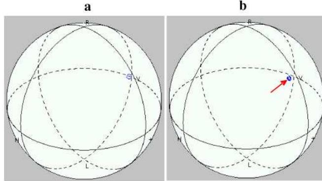
Fig. 9. PER measurement results: (A) PER measurement result with low stress on output FC/PC connector. (B) PER measurement result with relatively high stress on output FC/PC connector. The corresponding PER of light in the PM fiber is 39.6 dB; however, the PER of the output light is reduced to 31.1 dB due to stress induced birefringence. The deviation of the SOP evolution circle from the equator can be used to indicate stress induced birefringence at the exit end of the PM fiber.
