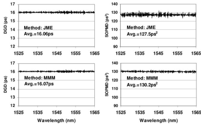
Fig. 5. DGD and SOPMD measurement results for a PMD artifact made from two 16 mm long YVO<sub>4</sub> crystals with a relative orientation angle of 45 degrees. (A) and (B) DGD values vs. wavelength obtained using JME and MMM methods, respectively. (C) and (D) SOPMD values vs. wavelength obtained using JME and MMM methods, respectively.
